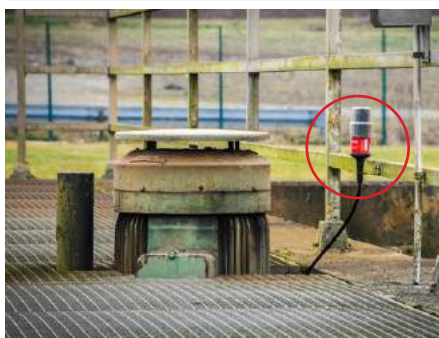
Lubrication of bearing at surface aerator
