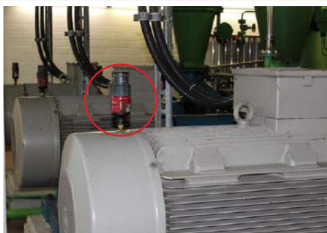
Electric motor bearing lubrication
