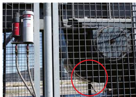
Lubrication of pillow block bearing on conveyor
