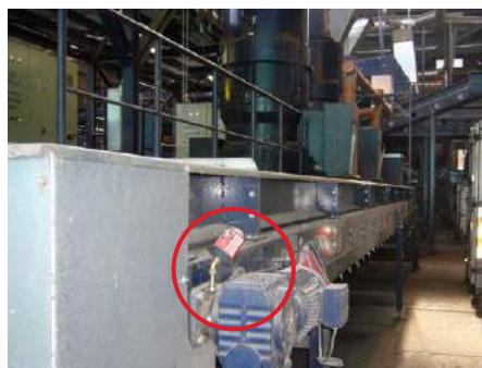
Lubrication of flange earring on conveyor
