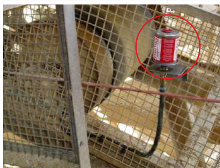
Lubrication of pillow block bearing on conveyor
