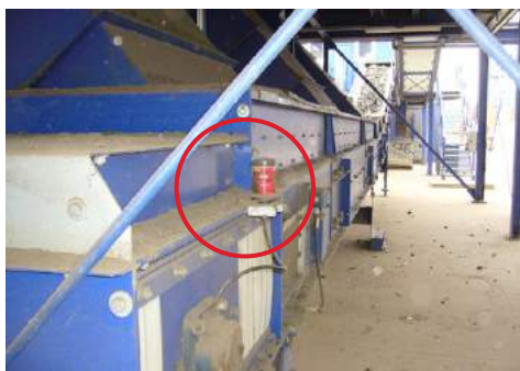
Lubrication of pillow block bearing on conveyor
