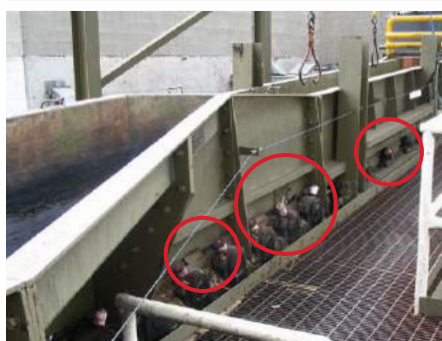
Bearing lubrication at the tree sorting system
