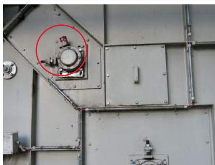
Lubrication of flange bearing on bucket conveyor
