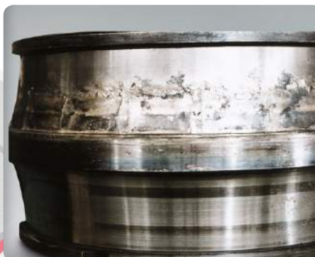
Bearing damage caused by lubrication starvation
