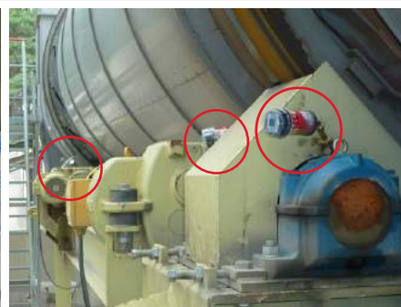
Lubrication of pillow block bearing on rotary dryer
